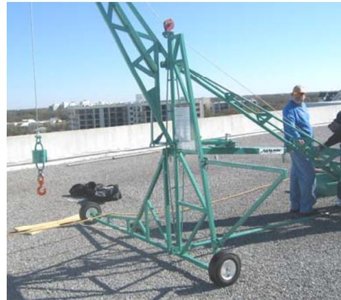
Fig 20. CAREFULLY roll Hoist into its' working location at the Roof Edge.
