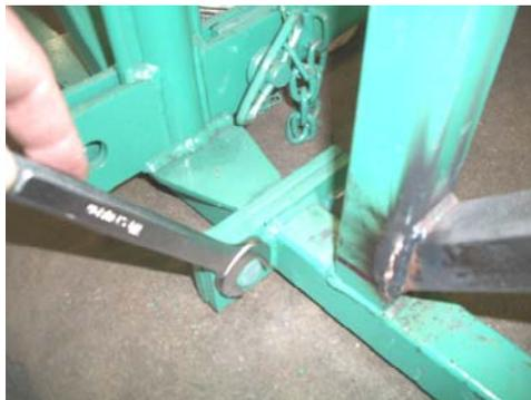
Figs. 2 and 3. Bottom of A-Frame to Side Leg. Use 3/4 inch Combination wrench or Crescent to tighten (2) 1/2 inch Bolts.
