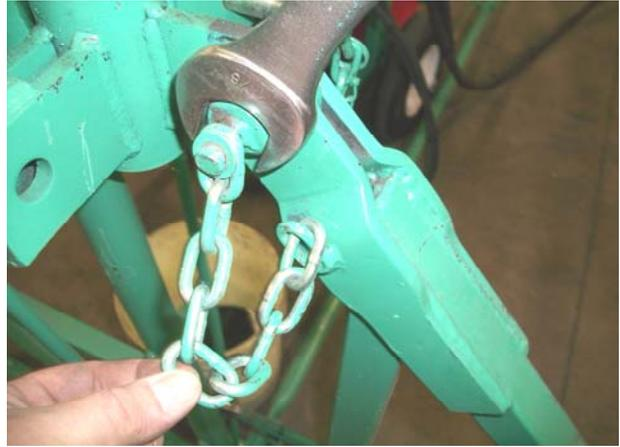
Figs. 4 and 5. Top of A-Frame to Side Leg. Use 1-1/8 inch Combination wrench to tighten 3/4 inch Bolt and Nut.
