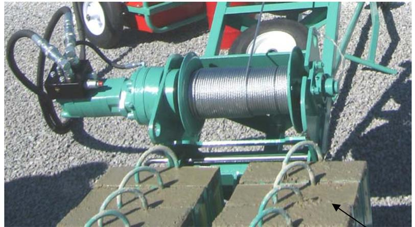
Figs 23 and 24. Install empty Counterbalance Pan onto back of Hoist. Place it so channel in bottom of Pan slips over rectangular Tube on back of Hoist. Slide Pan forward until holes in bracket align with holes in Boom and secure Pan in place with Pin and Clip attached to Pan. Load 16 concrete-filled Garlock Counterweights into Pan as shown.
