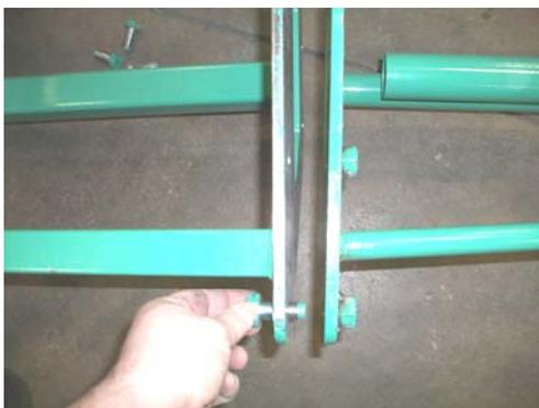
Fig. 1. Lower Boom to Upper Boom. Use 15/16 inch combination wrenches or Crescent Wrenches to install and tighten the (6) 5/8 inch Bolts and Nuts.
