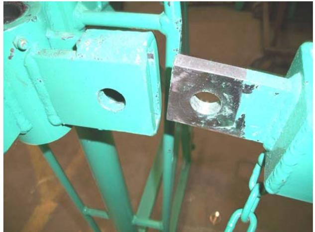
Fig 7: Insert front end of Antenna Brace into lower joint in A-Frame.
