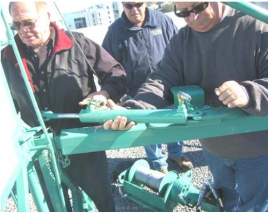
Fig 17. Install Swing Arm Cylinder as shown and secure in place with attached Pins and Clips. Note location of Winch Unit from previous step.
