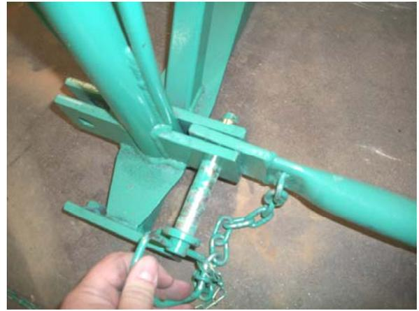
Fig 11. Insert front end of Lower brace into Joint on Bottom of A-Frame and secure with attached Pin and Clip. **Make sure to tighten T-Bolts on Lower Brace to hold it at the desired length.**
