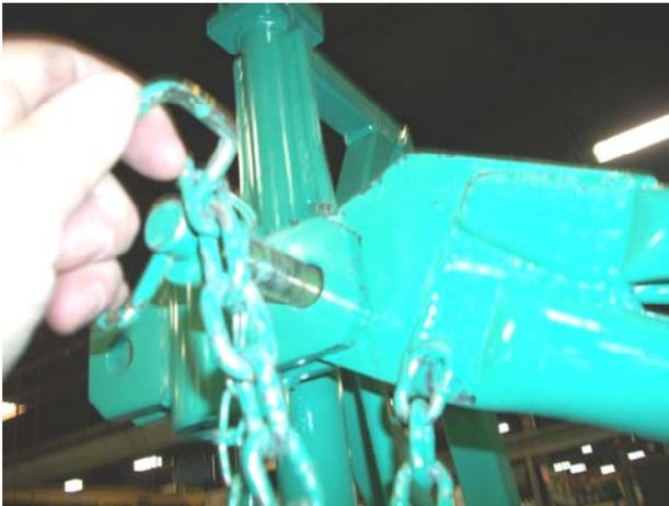
Fig 6: Lift Boom to upper Joint in A-Frame and Pin
