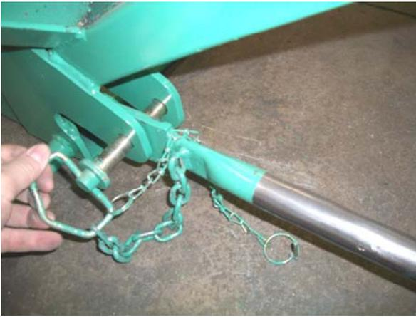
Fig 10. Insert back end of lower Brace into Joint on bottom of Boom and secure with attached Pin and Clip.
