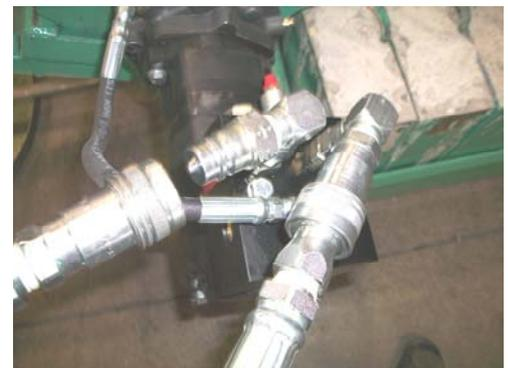
Figs 25, 26 and 27. Re-Install Power Unit Hoses (the large ones) onto the Winch Unit as Shown. Install the 2 smaller Power Unit Hoses to the Swing Arm Cylinder. Due to the different Fittings on each Hose, they only attach one way.
