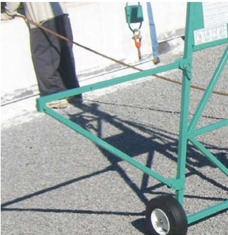
Fig 19. Lower the Operator fence into position. Remove Pin that holds Fence in the "stowed" position. Lower the Arm until hole in end of Arm aligns with holes in Upper Bracket and secure Arm in place with Pin.
