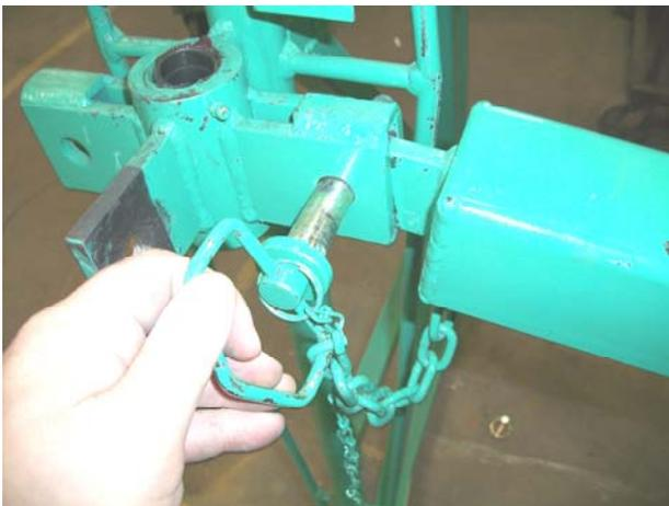
Fig 8. Secure Front end of Antenna brace to A-Frame using attached Pin and Clip.
